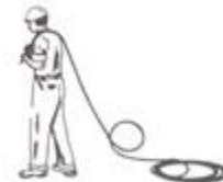
Do not pull out of a coil. Do not throw loops off a reel .
